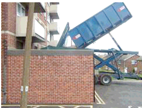
Figure 3: Delivery of biomass to a central store
